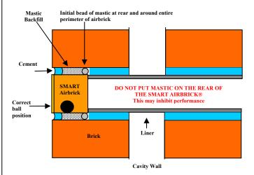
Mix sand and cement (PVA can be added to improve adhesion). Once the mastic has cured point the SMART Airbrick® with cement. Ensure the cement does not cover the front panel. Point the mortar to match the style of the wall. Remove masking tape.
